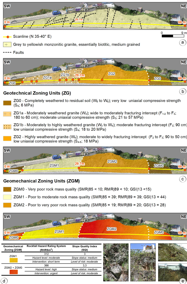
Figure 5: Geotechnical and geomechanical assessment: geotechnical and geomechanical zoning (the dots mark the zoning units' boundaries) and rock slope hazard zoning based on rockfall rating system and slope quality index. (a) Scanline and geological cross-section; (b) Geotechnical zoning; (c) Geomechanical zoning; (d) Rockfall hazard features; (e) Several aspects of the rocky slope instability.
